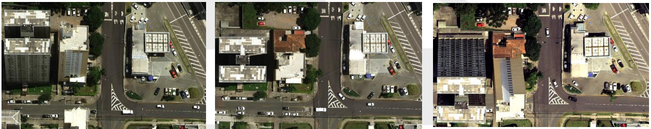
Backward (19°), Nadir (0°) and Forward (26°) RGB images from one of the first flight strips with ESTEIO's ADS100 sensor – Curitiba
